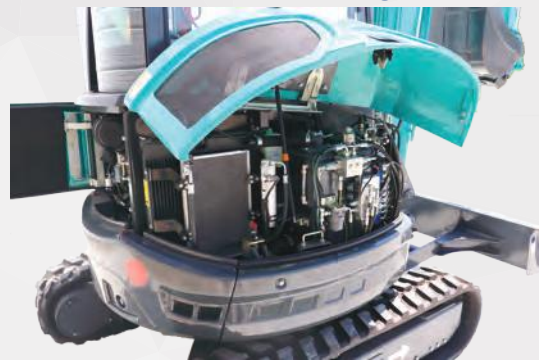
Kubota Engine with easy access panels for maintenance
