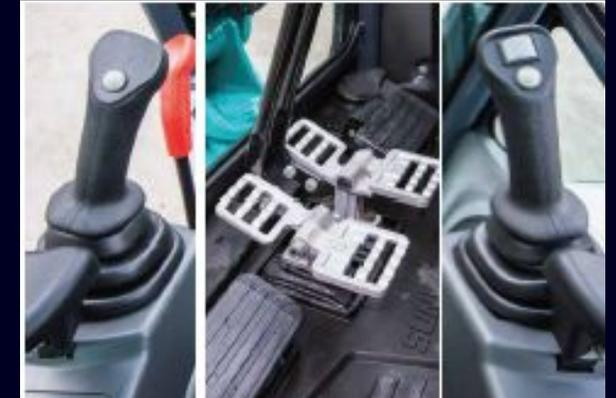
Equipped with electrical proportional joystick
